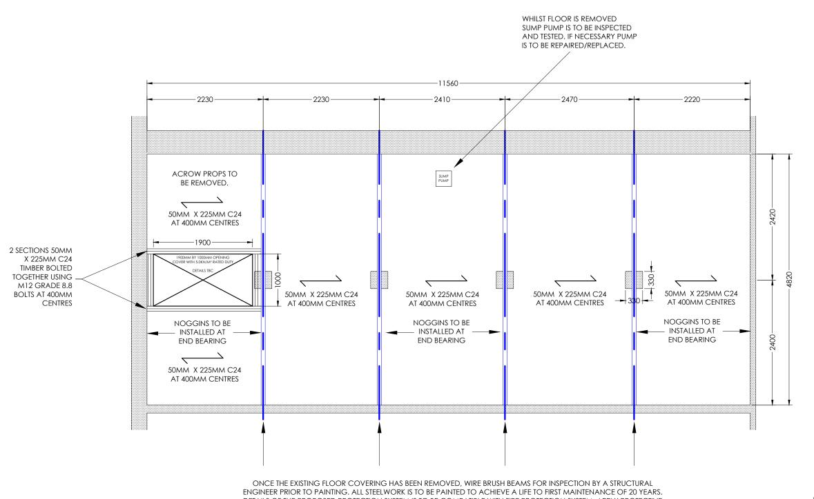
REMOVE ANY EXISTING DECAYED OR FAILED TIMBER JOISTS AND REPLACE WITH 50MM x 225MM C24 TIMBER JOISTS AT 400MM CENTRES.
